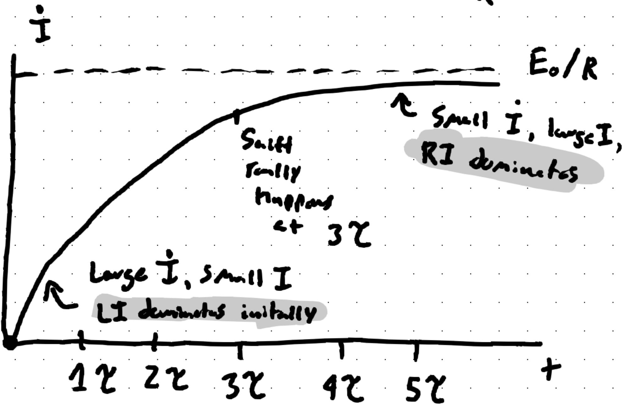
So initially, the total voltage is being used by mostly the inductor!
